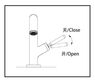
•The moving angles of the handle range from 0 to 22 degrees.
