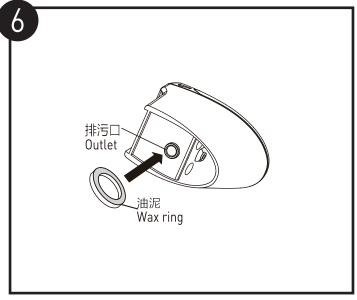
将油泥安装在陶瓷底部排污口上,注意连接紧密。 Install the wax ring on the drain outlet at the bottom of the ceramic, paying attention to the tight connection.
