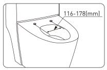
安装孔距离116-178mm之间 The distance between mounting holes is 116-178mm
