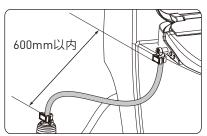
左侧距离角阀600mm以内 The left side is within 600mm of the Angle valve
